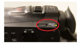
If the camera screen (small LED) is dark, check 3 cables going into the camera. Also, make sure the camera is on by checking the green light next to the On/Off button.
