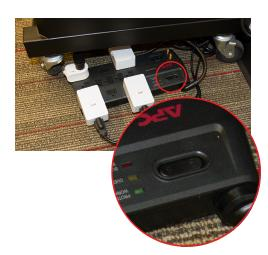
Most problems with the OBS system can be fixed by turning the entire system Off and back On using the power switch on the surge protector underneath the black cart.
